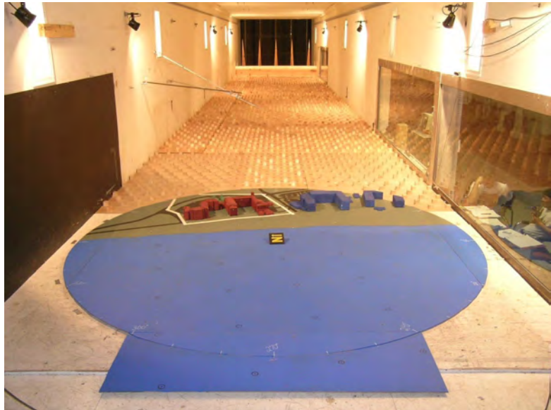
Figure 5: The suburban easterly flow approaching the resort buildings. These buildings are about 30 metres tall in full scale and they locally reduce the mean windspeed at sail height and add gustiness to the ambient conditions close to shore.
