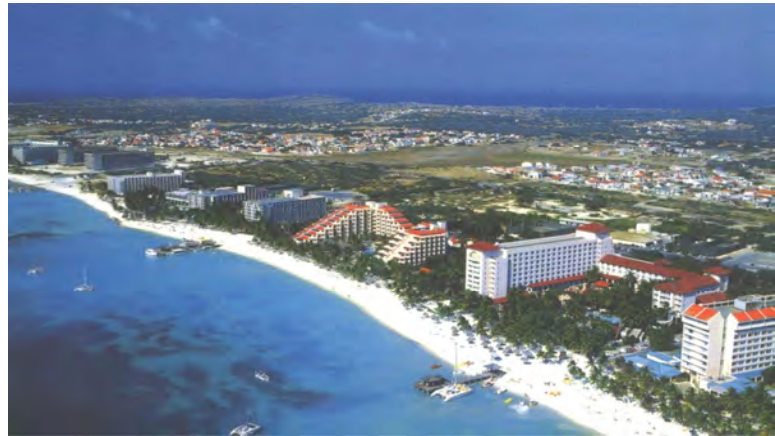
Figure 2: The randomly spaced taller buildings in Aruba are along the northwest Palm Beach coast. Sailing off the beach appears influenced by their presence to a distance of about 300 m offshore.
