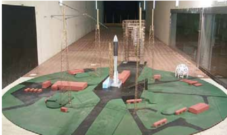
Figure 8: Aeroelastic model of the Titan V Launch Vehicle with the Mobile Service Tower backed away to the rear.
