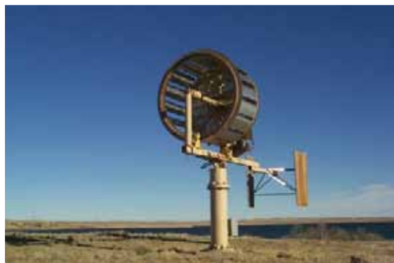
Figure 17: Full-scale wind turbine design is used to confirm model studies in the wind tunnel and initial CFD input.
