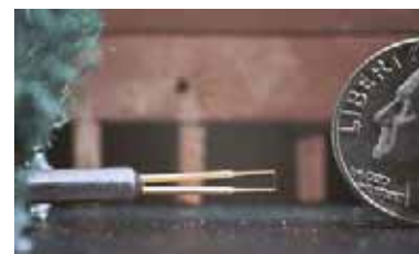
Figure 2: The hot-film anemometer has traditionally been used to collect turbulent velocity data in the wind tunnel.
