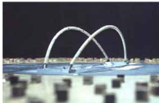
Figure 9: Aeroelastic model of the Galleria Arches in Houston, Texas.
