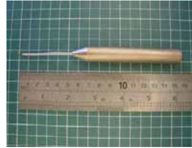
Figure 3: Four-hole Cobra probe in use at HKUST (after Dr. Peter Hitchcock).
