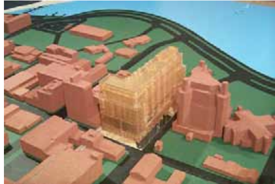
Figure 10: Simultaneous pressure data collection applied to a midrise condominium in Miami (510 taps).
