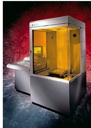
Figure 1: The laser booth and operational console of a stereolithography machine.
