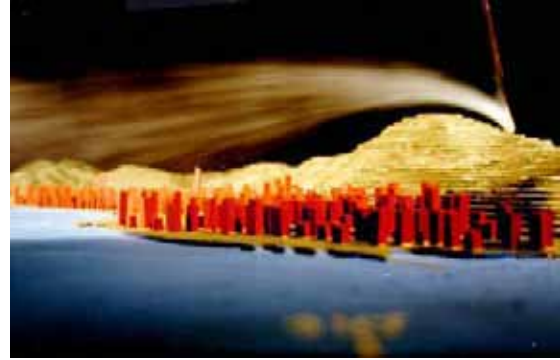
Figure 18: Separated flow over Central caused by southerly winds over Victoria Peak in Hong Kong, China (1:4000).
