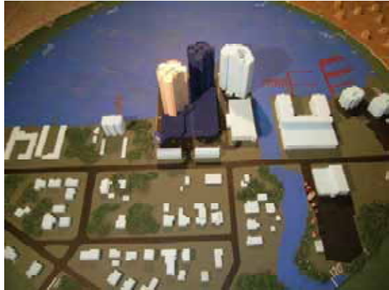
Figure 13: Thirty-storey Florida condominium, with tall proximate neighbours, used to compare balsawood HFFB (shown) data with the simultaneous pressure technique.
