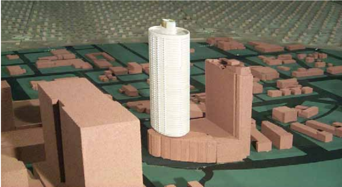
Figure 21: The oval building in the centre generated large torsional loads on the rectangular building to the right by partially shielding the dominant winds on its wide face. Fortunately it was tested with and without the oval building in place during a previous study and was designed to accommodate the torsional loads. How many buildings are not assessed in this manner?
