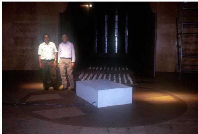
Figure 6. The 1:10 TTU Building model in the large Monash University wind tunnel (after John Holmes).
