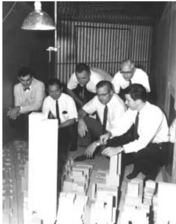
Figure 3: Testing the World Trade Center Towers in 1964 in a boundary-layer wind tunnel at CSU. The people are (left to right): A.G. Davenport, M. Yamasaki, M. Levy, J. Skilling, J.E. Cermak and L.E. Robertson (Colorado State University archives).
