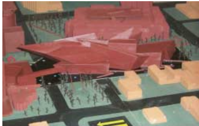
Figure 4: The Denver Art Museum is a non-typical shape, and applying a code procedure is inadvisable (after CPP Inc.).
