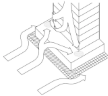
Figure 6: The tower-on-podium massing often results in reasonable conditions at ground level, but the podium may not be useable.
