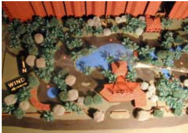
Figure 19: A detailed multi-phase study of a beachside hotel complex (pools, putting green, restaurant/bar etc.) with porous screens and extensive foliage.
