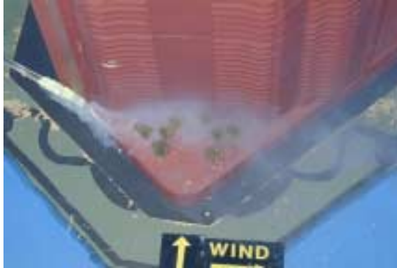
Figure 17: Accelerated flow around a tower corner washes over a pool deck.
