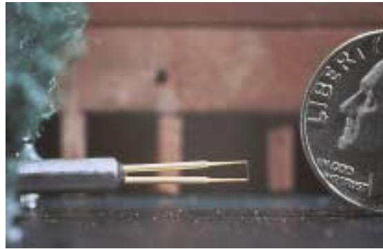
Figure 12: The hot-film anemometer uses variations in electrical resistance, induced by cooling due to airflow, to measure mean and peak wind speeds in the boundary-layer wind tunnel.
