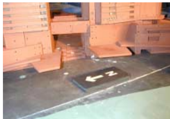
Figure 16: Horizontally accelerated flow between two tall towers may be minimized by judicious orientation away from dominant winds.
