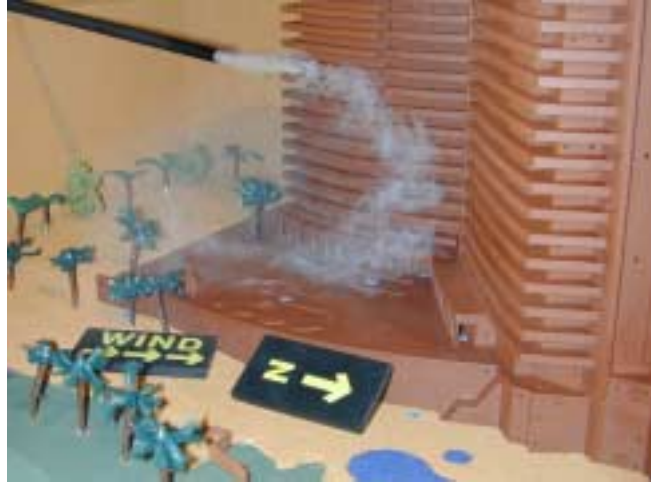
Figure 1: Downwash circulates over the podium pool deck of a 1:300 wind-tunnel model of a beachside condominium. This circulation requires ameliorative measures like an open trellis and substantial foliage.
