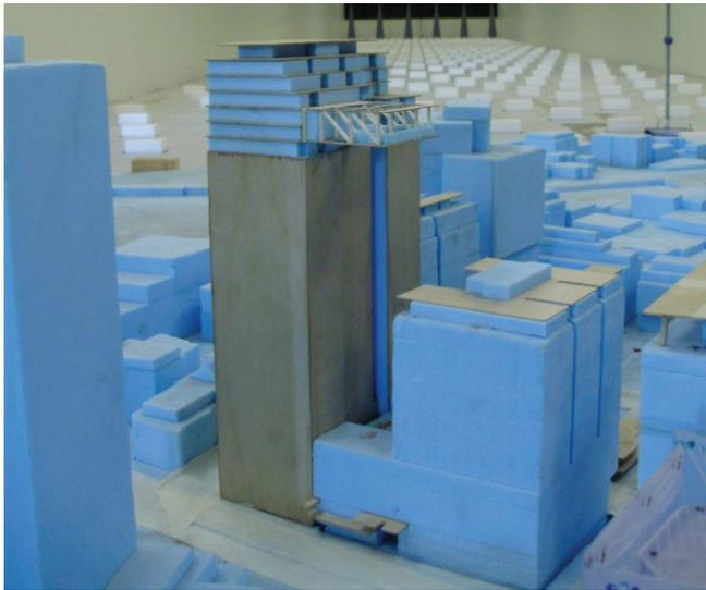
Wind tunnel testing 1:400 scale tests.
